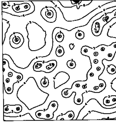
Figure 5.9: Simulated iron ore deposit — kriged standard deviation map for the kriged contour map from random samples.
